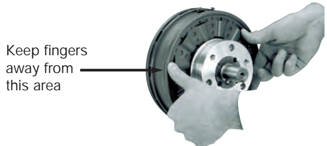
Figure 6 - Setting the airgap
