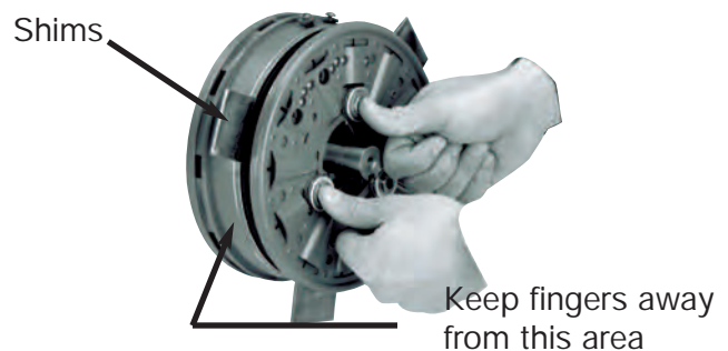
Figure 10 - Armature installation with shims in place.
