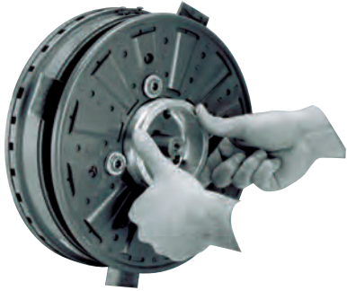
Figure 17 - Setting the airgap.
